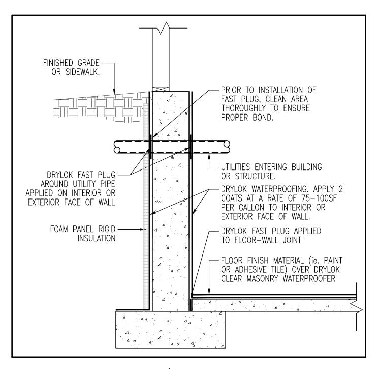
DRYLOK CONCRETE/MASONRY WATERPROOFER
